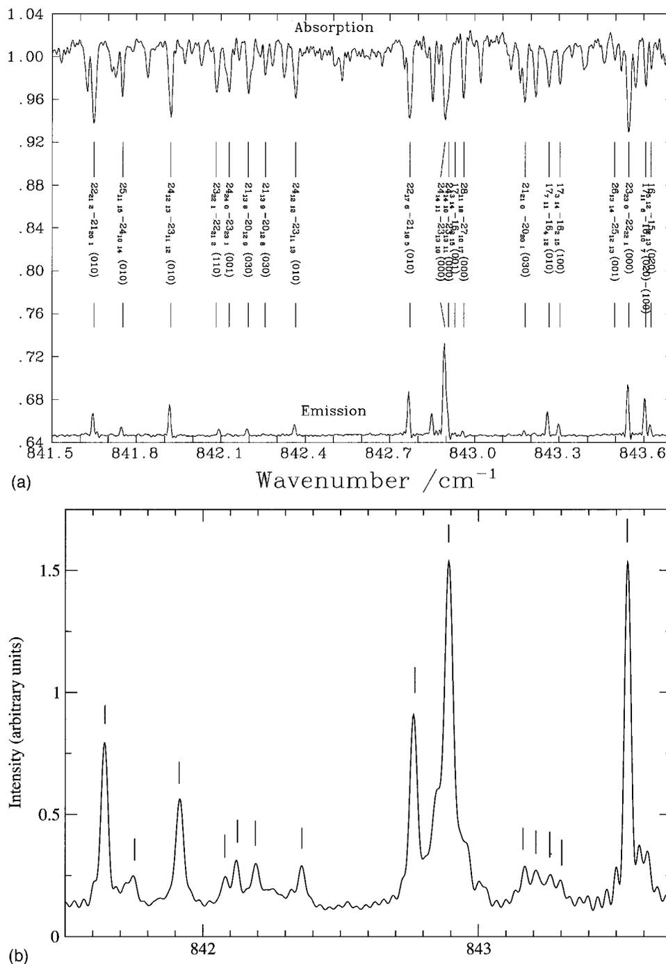
FIG. 3. Upper panel: sunspot absorption (upper trace) and laboratory emission from heated cell spectra (lower trace) from work (Ref. 30) near 840 cm<sup>-1</sup>. Lower panel: torch spectrum in the same region; vertical lines denote assigned transitions.
