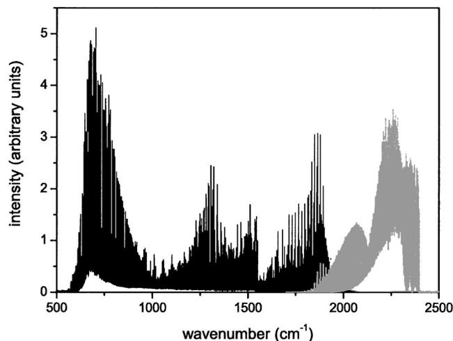
FIG. 1. Raw emission spectrum of the oxy-acetylene flame in the  $500\text{--}2500\text{ cm}^{-1}$  spectral region.
